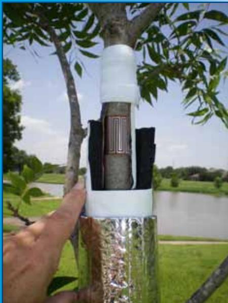
EXO Sensor showing the different layers of insulation and shielding that comes with each sensor.
